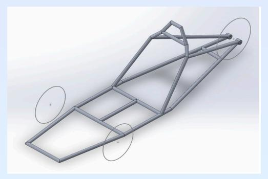
Models were designed on SolidWorks and analyzed using FEA analysis to ensure the designed and selected frame would be sufficient for the maximum load applied once completed.
