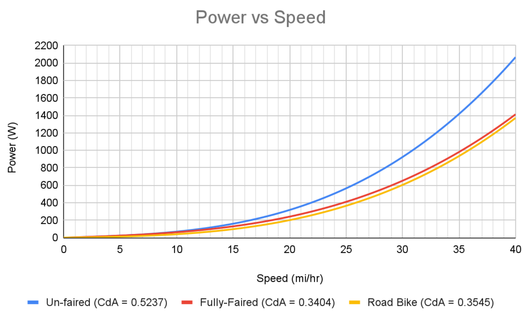
Figure 2: Power vs Speed of Road Bike vs Faired and Un-Faired Trike
