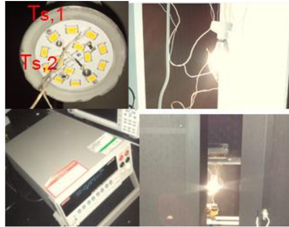
Fig.4 T_s measurement with thermal couples
