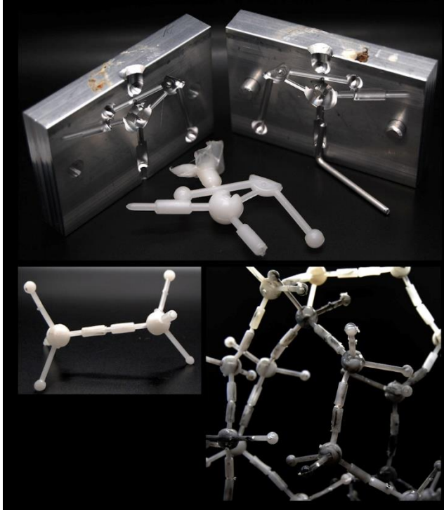
Figure 1. A custom aluminum injection mold that creates a ball-and-stick model of polyethylene
